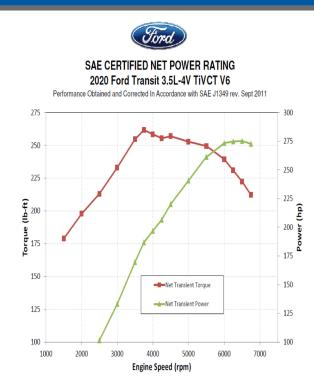
SAE Advertised Performance with Regular Fuel 262 lb-ft at 3750 RPM 275 hp at 6500 RPM
