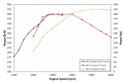
SAE Advertised Performance with Regular Fuel 400 lb-ft at 3000 RPM 325 hp at 5000 RPM
