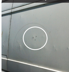
Outward dents to panel
