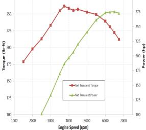
SAE Advertised Performance with Regular Fuel 262 lb-ft at 3750 RPM 275 hp at 6500 RPM
